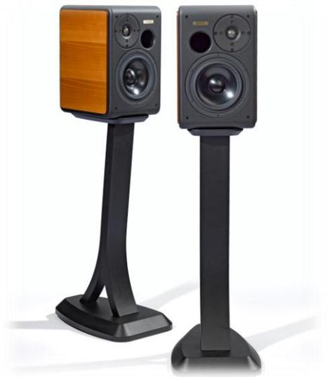
Prima uses the same one-inch Scanspeak tweeter that features throughout the *Classica Series* because of its first-class characteristics. It's an extremely solid and powerful soft-dome design that boasts a large decompression chamber and a well-measured use of ferrofluid to cool and centre the voice coil. The tweeter has been specified for 1mm (peak-to-peak) linear excursion, ensuring outstanding power handling as well as very low harmonic and inter-modulation distortion.
