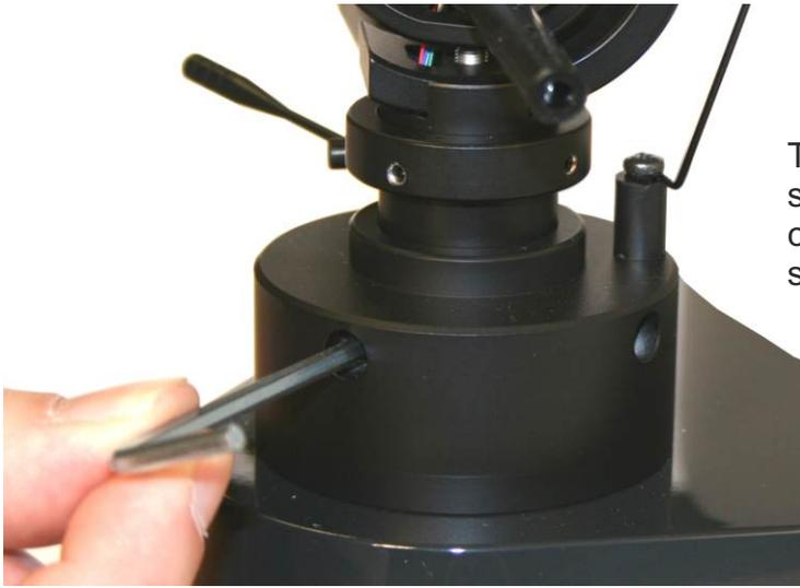
This picture shows how the arm pillar slides up and down through the support collar and is locked in place by the allen screws.
