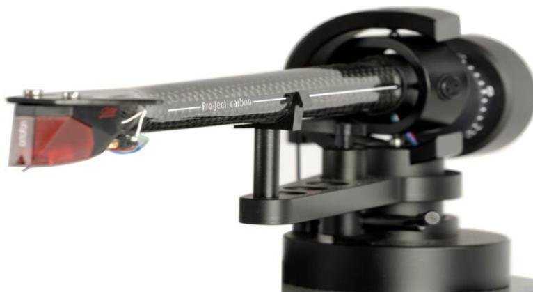
Pro-Ject has met this requirement superbly on most of its turntables by using a carbon fibre tube, which is one piece from pivot to the cartridge mounting platform. In addition to being one piece, the carbon fibre arms are almost completely free from flexing, by virtue of the fibre alignment, and through their conical tube shape have a high order of rigidity and a freedom from the 'tube resonance', which can degrade the performance of conventional arm-tubes.
