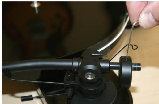
Carefully move the counterweight along the rod away from the bearing to add more pressure or towards the bearing to reduce the pressure. During this process keep lifting the stylus away from the gauge in order to prevent any damage to the stylus.
