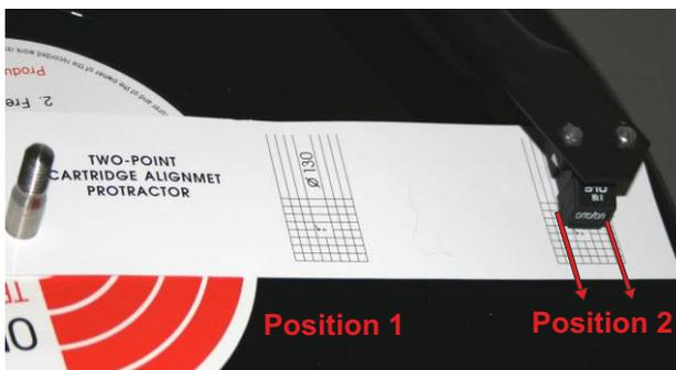
The Alignment Card should be fitted over the centre spindle and laid flat on top of a vinyl disc. As shown in this picture there are two calibration points, one near the centre of the disc and one near to the outside edge.
