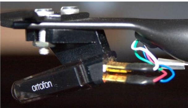
Now fit the four coloured wires to the pins on the cartridge as shown. The cartridge will normally have its pins colour coded the same as the wires but in other cases follow the following code:
