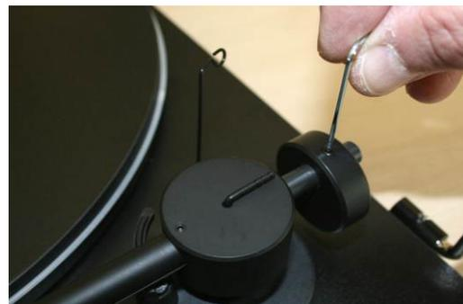
Once the gauge is balanced you should lock the counterweight into position using the hexagonal key provided.
